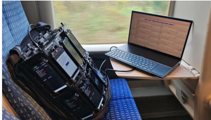
Figure 2: Train test setup - with technician computer and smartphone backpack.
